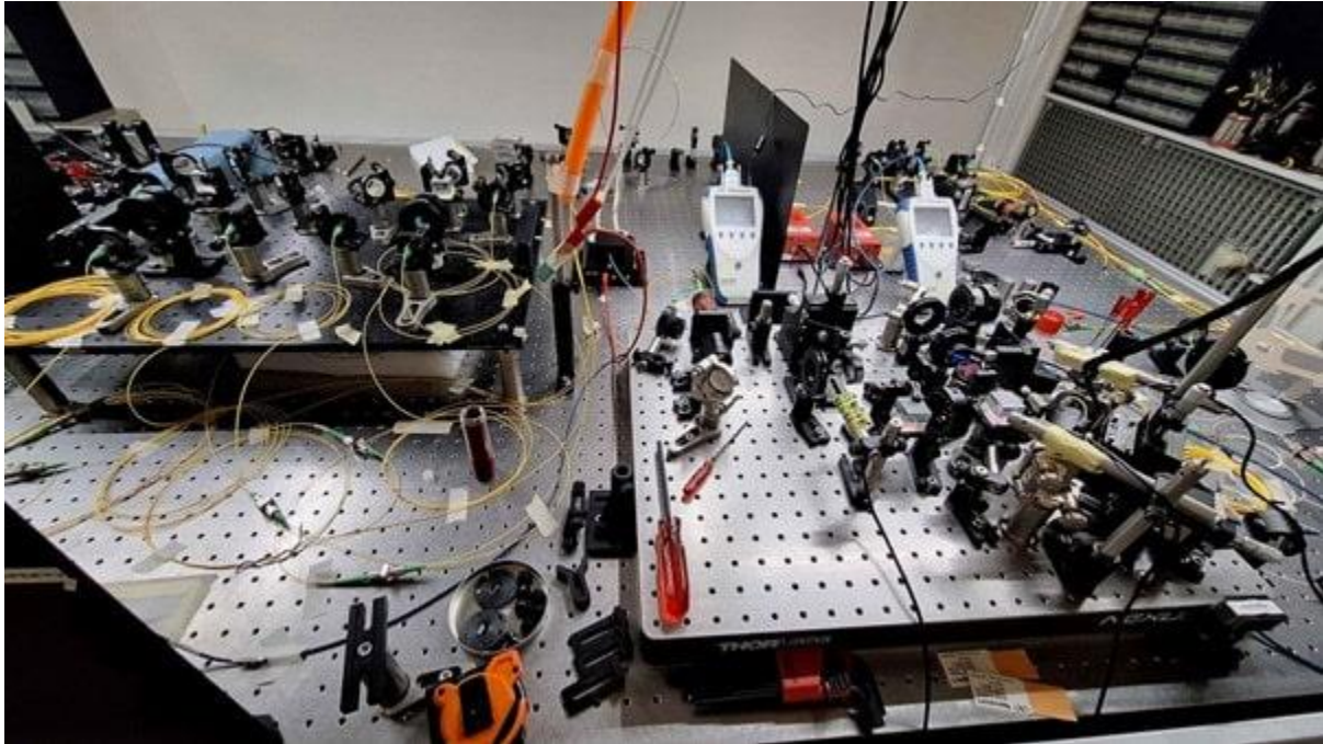
Figure 6: Photo of the optical setup for the type-0 source . It consists of a pump laser (blue fiber on the bottom left), a Type-0 Sagnac source (optical breadboard on the right), analysis stage (on the left) and a DWDM (white box under analysis stage).
